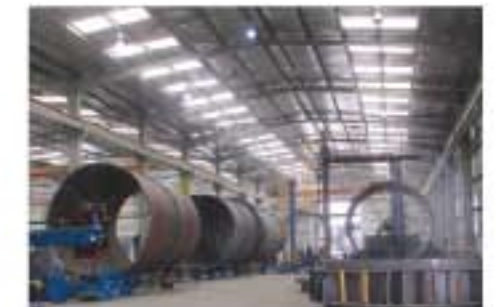
Exhaust stack fabrication and assembly line
